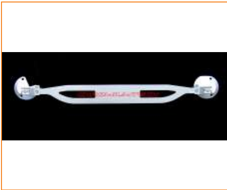
BMW E46 3-Series Aluminium Rear Upper Strut Brace Bar
